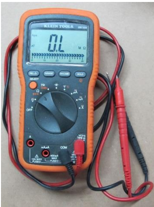
The multi-meter (left) has a resistance setting to measure ohms. This is a typical type of (megohm) measuring device capable of applying voltage to an in-ground loop.
