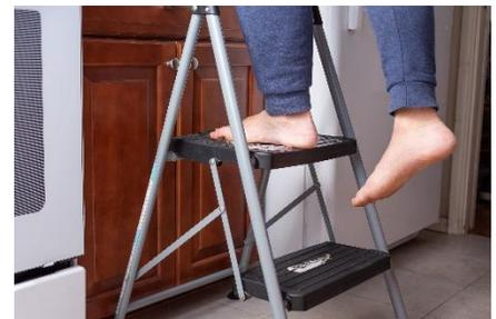
aluminum ladders is electrical conductivity. Aluminum is an excellent electrical conductor, while wood, unless completely saturated with water, generally is non-conductive.
